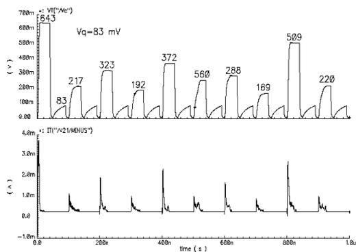
Figure 2 Fault-free multiplier response
