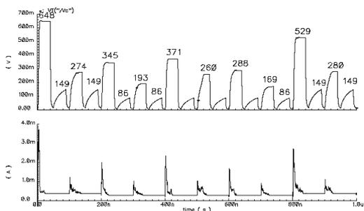
Figure 3 Multiplier response in a presence of a shot fault
