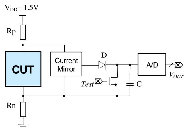
Figure 1 Dual-Resistor Current Monitor (DRCM)
